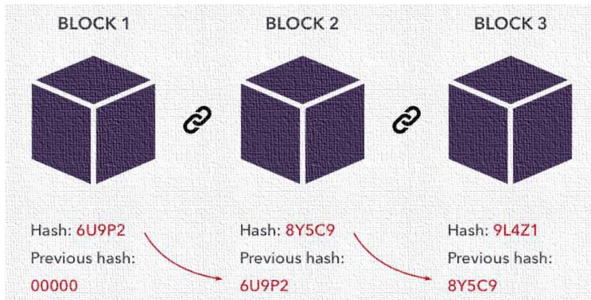
Figure 1. Structure of a Blockchain
